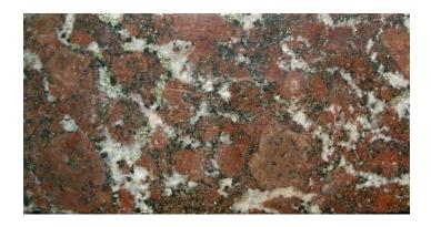
Magnetite, carbonate, biotite with economic chalcopyrite and minor pyrite mineralization. (From Ernest Henry rock type collection.)
