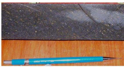
Massive magnetite-chalcopyrite from the Salobo deposit.
